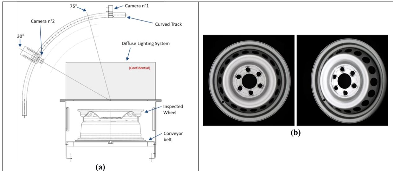
**Figure 2: a) Illustration of the AVI prototype installation, b) example of acquired images with two cameras.**
