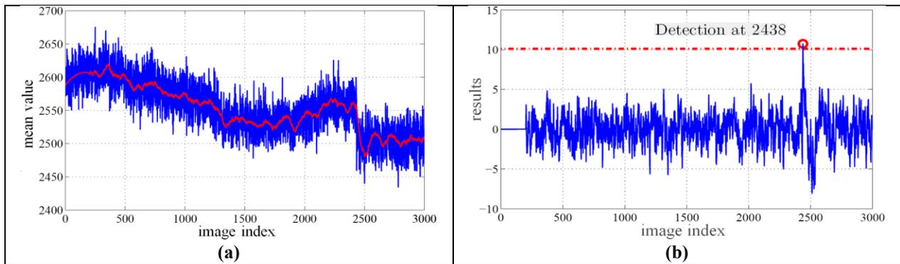
Figure 4: a) Real example of the variation of mean value with a change point at index 2434 and b) the detection result with the proposed sequential method for a maximal detection delay of 5 wheels.
