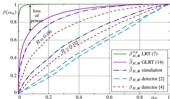
**Fig. 3:** Detection performance of LRT, proposed test and detectors proposed in [4, 5] for textured image.
